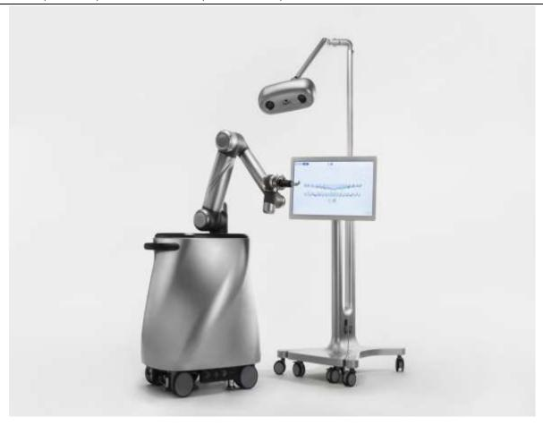
Passive robots: Robots such as Yomi (Neosis Inc., Miami, United States) and DentRobot (Dcarer Medical Technology Co., Ltd, Suzhou, China) require the operator to guide their robotic arms during the procedure. The operator is responsible for the robot's entry and exit from the mouth, preparation of the implant site, and placement of the implant.
